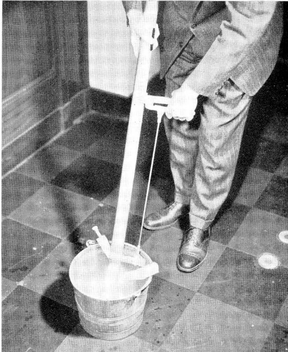
FIG. 146.—Apparatus known as a Bazooka used to destroy burnt-out Fluorescent Lamp Tubes under Water. This aims at the prevention of Beryllium Granuloma of the skin following cuts
