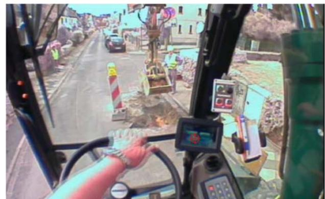
"Dikablis" mobile eye tracker for tracking of eye movements (top, source: Ergoneers GmbH, Manching). Tracking on board the excavator: the red cross-hairs on the monitor show the focus of the eyes (bottom).
