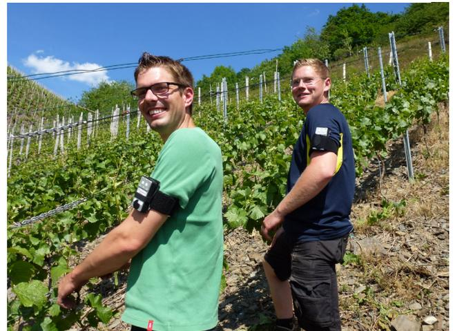
Vineyard workers during the measurement campaign, wearing the GENESIS-UV electronic data logger/dosimeter
