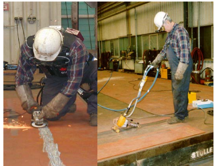
Processing welding seams with a hand-held angle sander (left) and the hand-guided belt sander (right)
