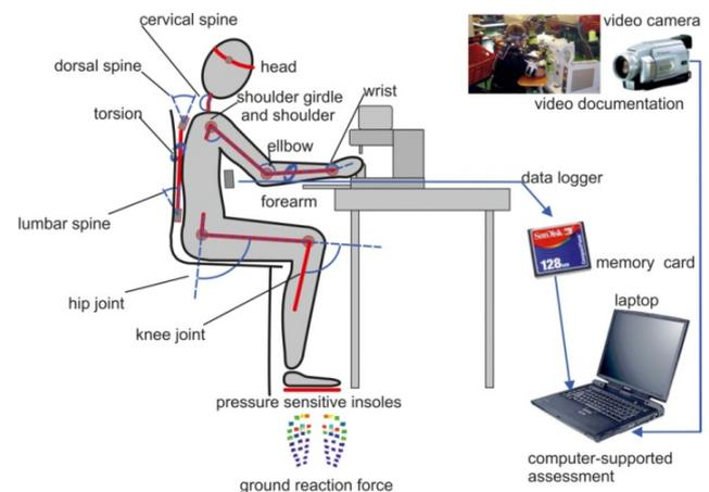
Schematic design of the system for recording bodily movement. Recorded shoulder-arm movements: shoulder girdle, shoulder joint, elbow joint, forearm, wrist
