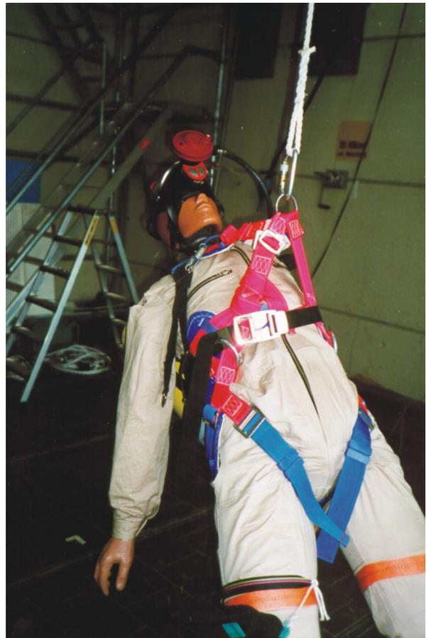
A dummy protected in a fall arrest system. The breathing mask was pushed up by the front harness hook such that the seating no longer provided an airtight seal. This also indicates the risk of injury to the face.
