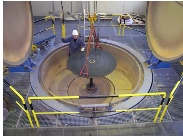
Centrifugal speed tester for centrifugal force tests involving grinding tools
