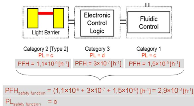
Figure 2: Linear combination of SRP/CS (with PFH-values) for the safety function „Stop actuator if light barrier is interrupted“.
