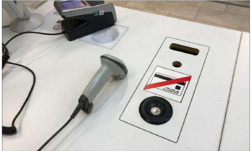
Figure 2: Magnetic hard label remover
