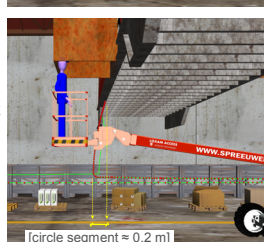
[Accident collision of operator with environment]
