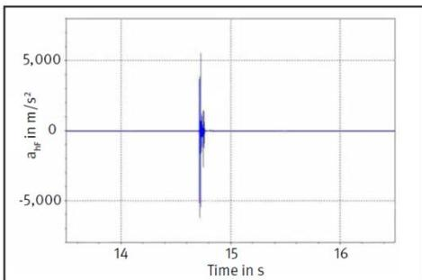
Figure 5: Time characteristic of the flat<sub>h</sub>-weighted acceleration
