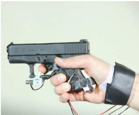
Figure 4: Pistol with sensor
