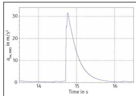
Figure 6: Time characteristic of the flat<sub>h</sub>-weighted running root-mean-square value
