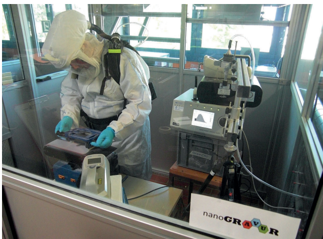
Figure 3a Workplace for sanding nanocomposite materials with a set of particle measuring instruments. Source: IFA
