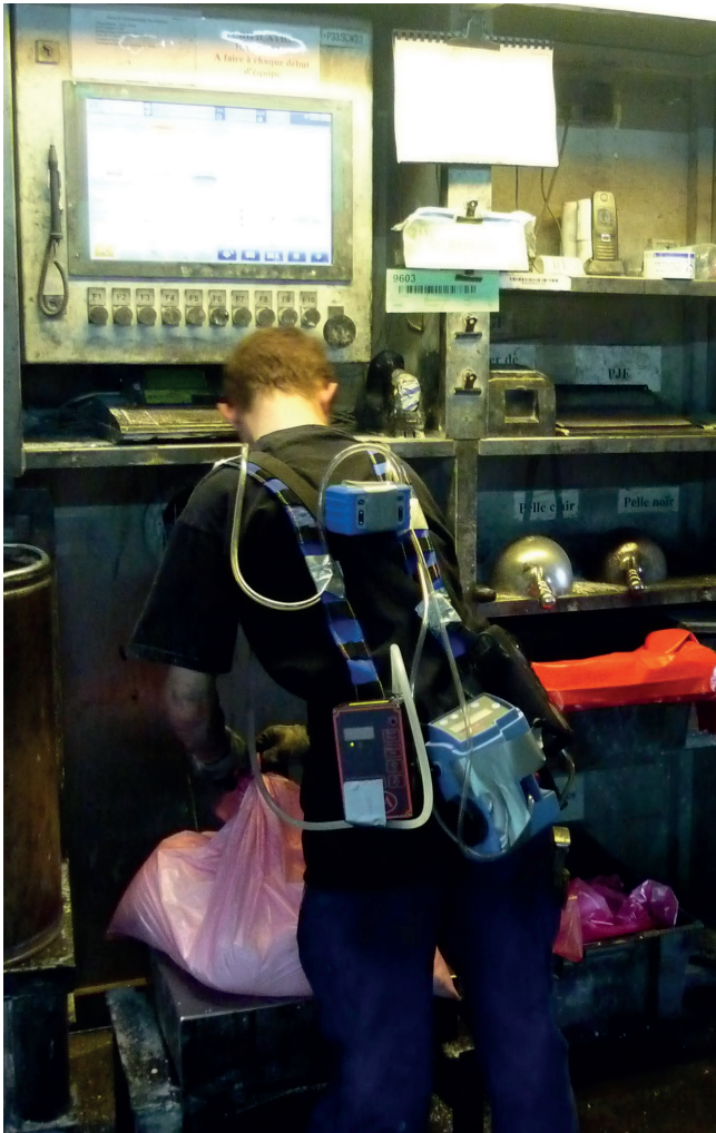
Figure 1 Weighing operation with an operator closing the weighed bag of powders at the workstation and carrying the real-time measuring instruments, including the DiSCmini. Source: ©INRS
