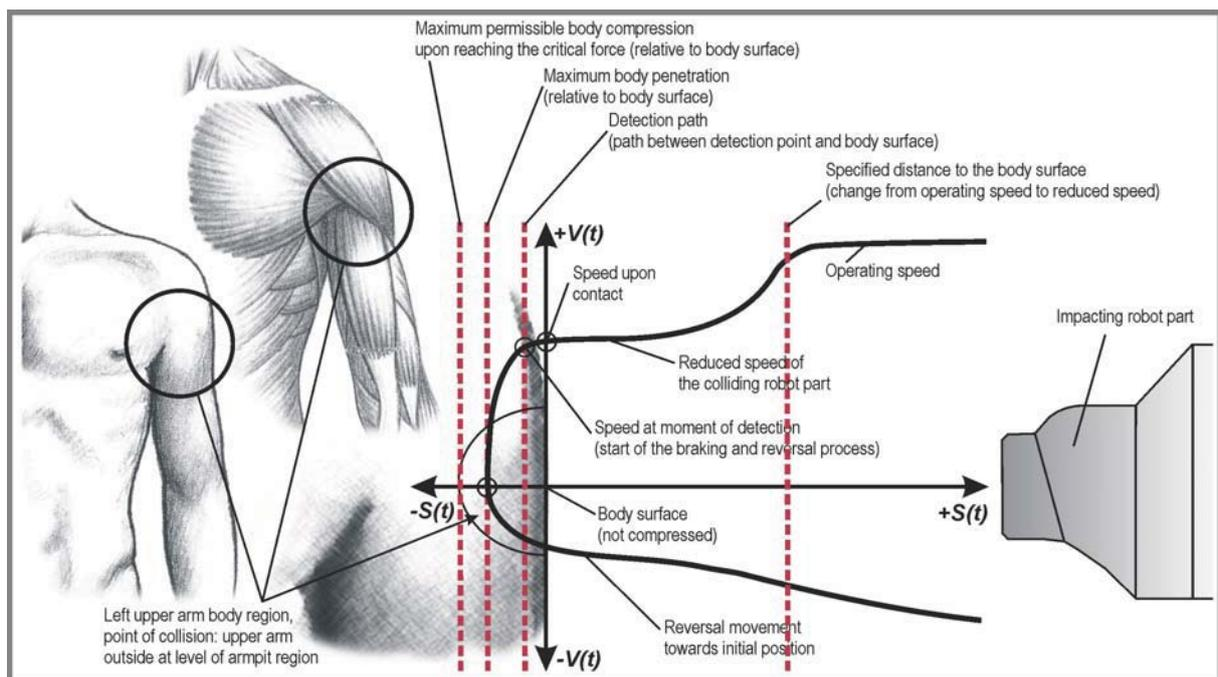
Figure 1: Kinematic process of a collision between a specific robot part and a human body; effected individual body region is the upper arm region – outside
