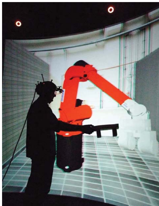
Figure 4. Experiment with simulated collaborating robot.
