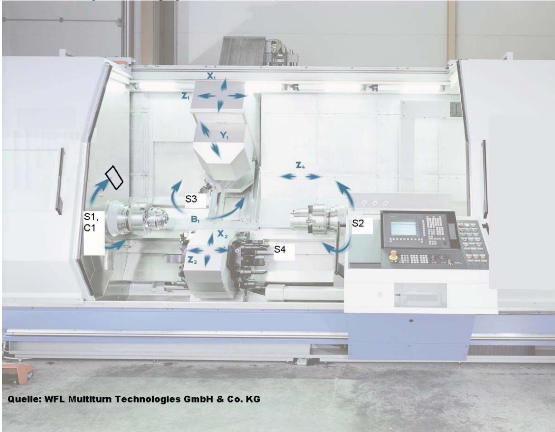
Figure 1: Scheme of axes of a machine tool. S_i, B_1 are rotations, X_i, Y_i, Z_i are translations, C is not considered (Source: WFL Multiturn Technologies GmbH & Co. KG, Austria, A-4030 Linz)
