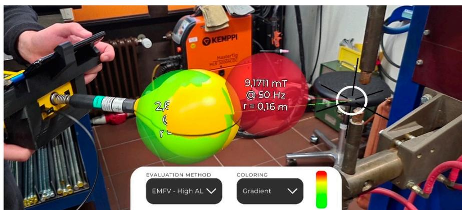
**Figure 5.** View of a measurement being taken as seen from the perspective of a second device. The virtual sphere representing the measurement coincides well with the measurement probe. The partial occlusion of the virtual sphere is possible due to the time-of-flight depth sensor in the smartphone.
