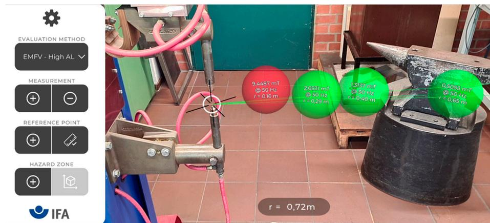
**Figure 2.** A typical measurement visualization regarding a resistance welding machine. The user interface on the left allows for the addition and removal of measurements (shown as colored spheres), or for the definition of a reference point (the white circle with the black axis). The coloring of the spheres indicates whether limit values are exceeded and depends on the selected evaluation method. The current distance to the reference point is shown at the bottom (e.g.,  $r = 0.72\text{ m}$ ).
