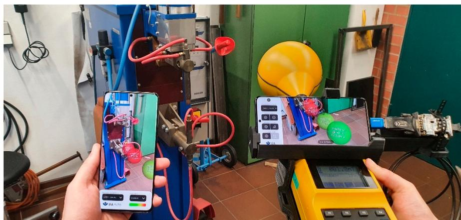
**Figure 4.** The Cloud Anchor functionality allows devices to share a common reference frame. By exchanging data about the objects in the scene, it becomes possible to view them independently from different perspectives with separate devices.
