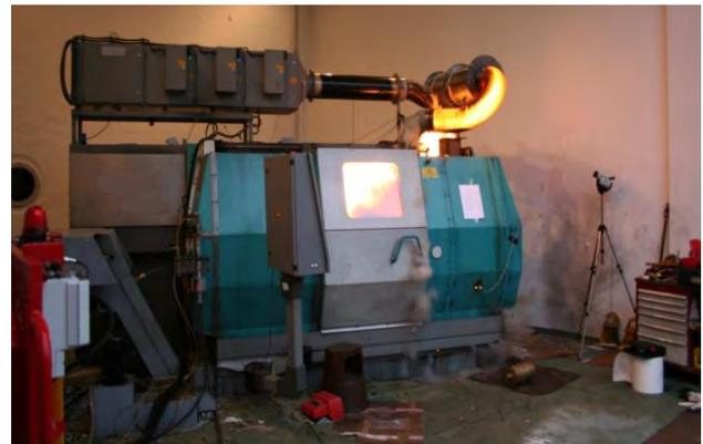
**Figure 2:** Flame propagation in the extraction
