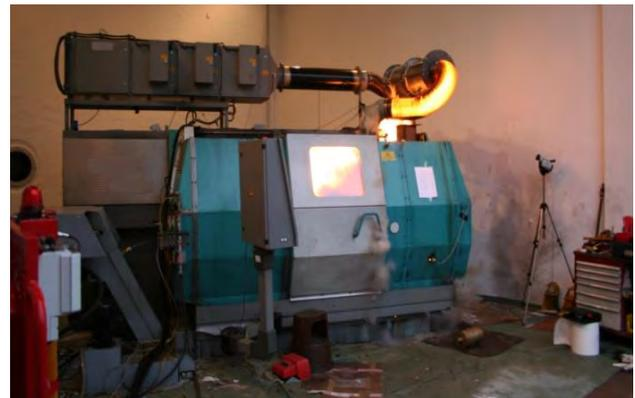
**Figure 2:** Flame propagation in the extraction
