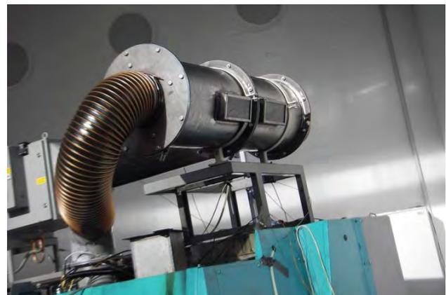
**Figure 3:** Flame arrester by INDEX/Büchel
