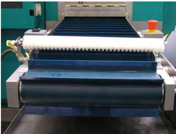
**Fig. 8:** Conveyor belt with crossbars, covered at the machine entrance
