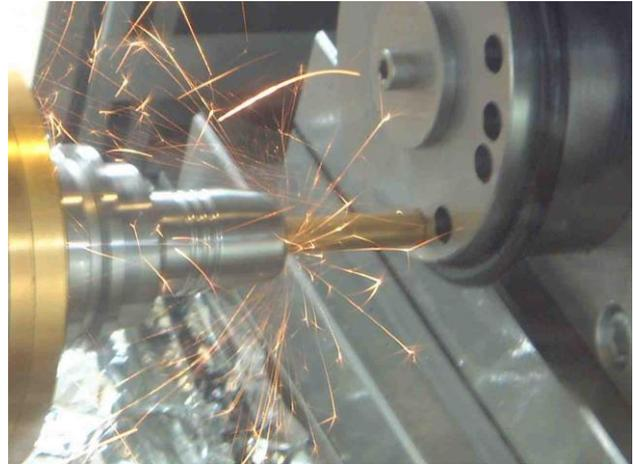
**Figure 3:** Ignition sparks during drilling
