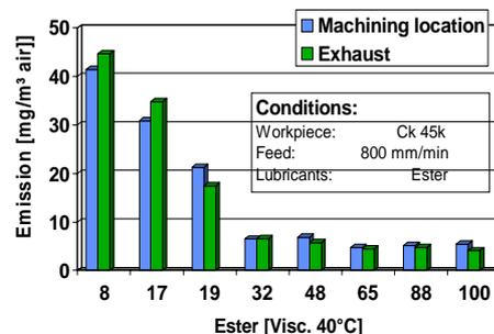
**Figure 3: Oil aerosol and oil vapour emissions at the cutting location**
