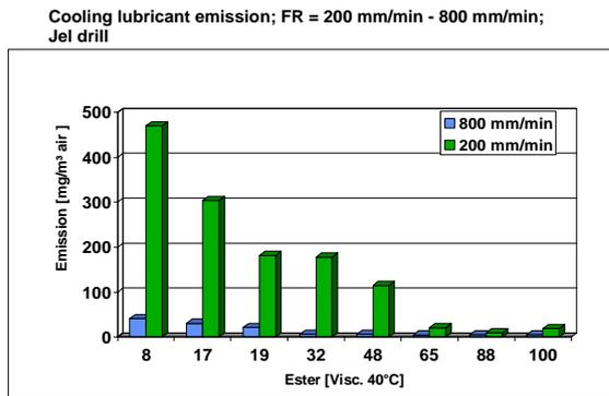
**Figure 4: Emission values of oil aerosol and oil vapour at reduced feed rate**
