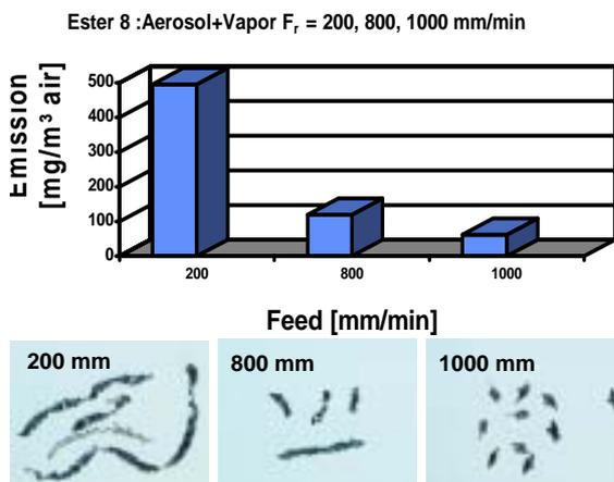
**Figure 5: Variation of feed rate when applying the lubricant ester 8 with formation of chip shape**
