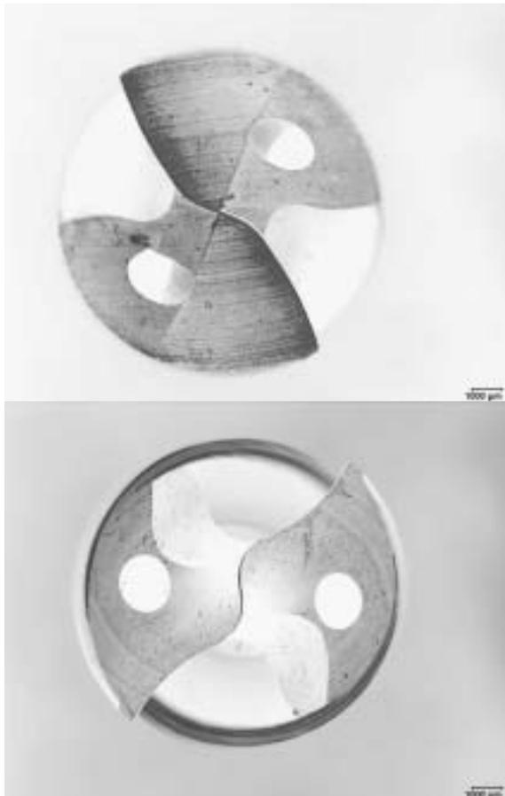
**Figure 2: Applied twist drills for the dry tooling in the front view**
