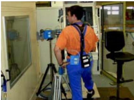
**Figure 8: Exposure measurements at persons and at the control panel**
