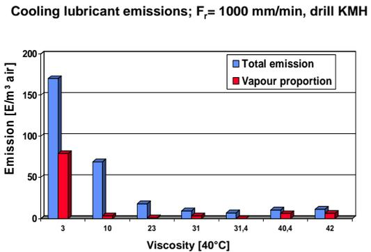
**Figure 6: Cooling lubricant emissions finished products; feed rate: 1000 mm/min**
