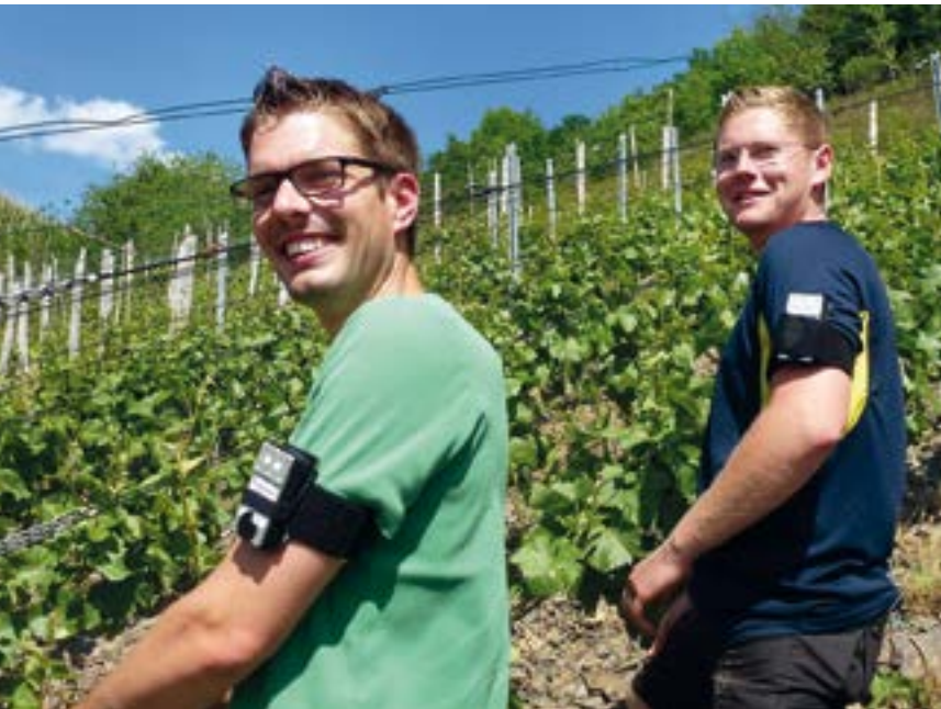
Measurement of UV radiation exposure during work in a vineyard
