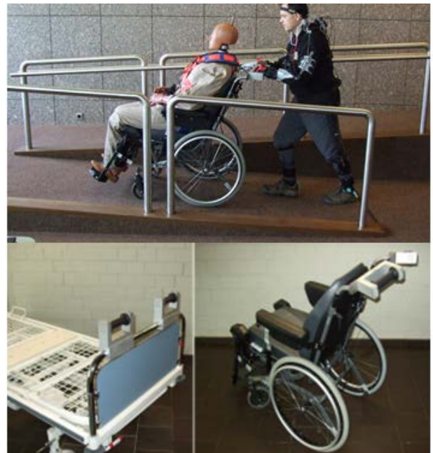
Body posture measurement system and dummy in a wheelchair during travel over a ramp (top). Force measurement handles on the bed and wheelchair (bottom)
