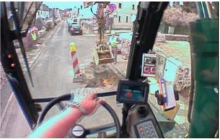
"Dikablis" mobile eye tracker for tracking of eye movements (top, source: Ergoneers GmbH, Manching). Tracking on board the excavator: the red cross-hairs on the monitor show the focus of the eyes (bottom).
