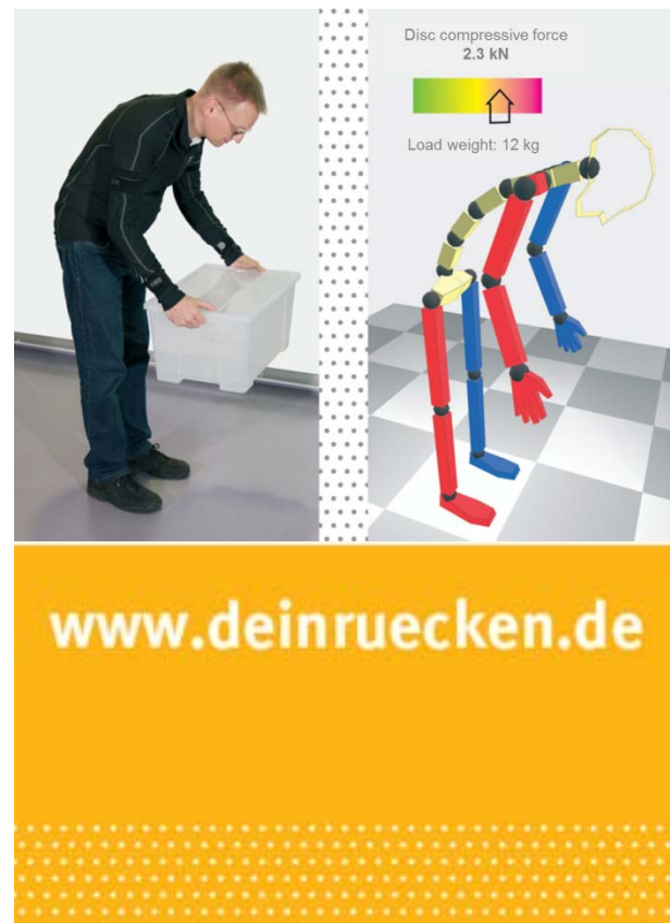
CUELA back monitoring system – test subject wearing sensor jacket, and virtual rendition
