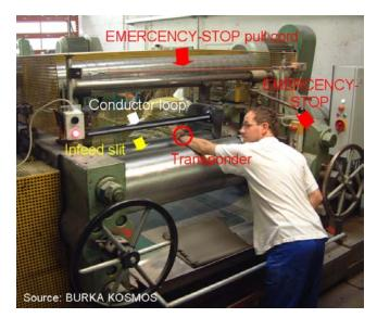
Safeguarding of danger zones: infeed slit on a calendering machine with horizontal roller arrangement in the abrasive materials industry (during trialling)
