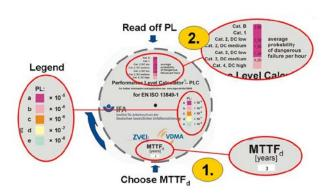
Use of the performance level calculator (two counter-rotating discs) for calculation of the PL in just two steps: select and read-off
