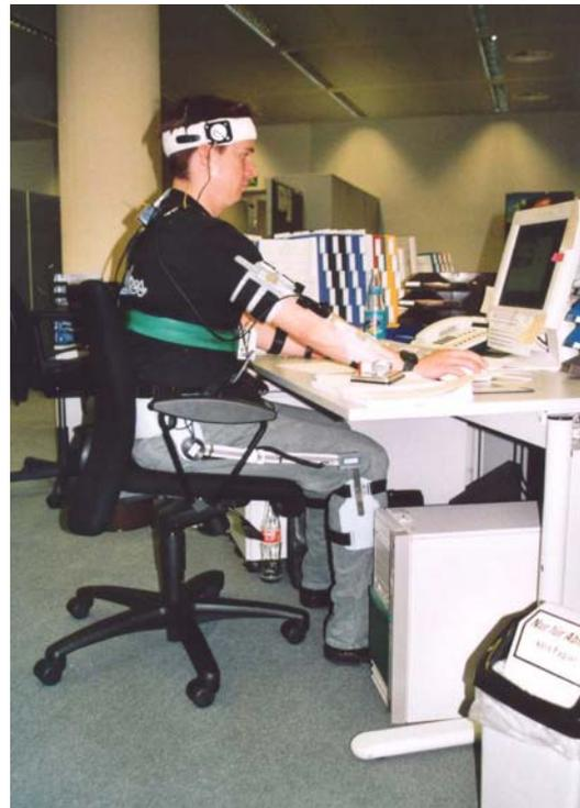
Posture measurements with the CUELA measurement system at a call-centre workplace
