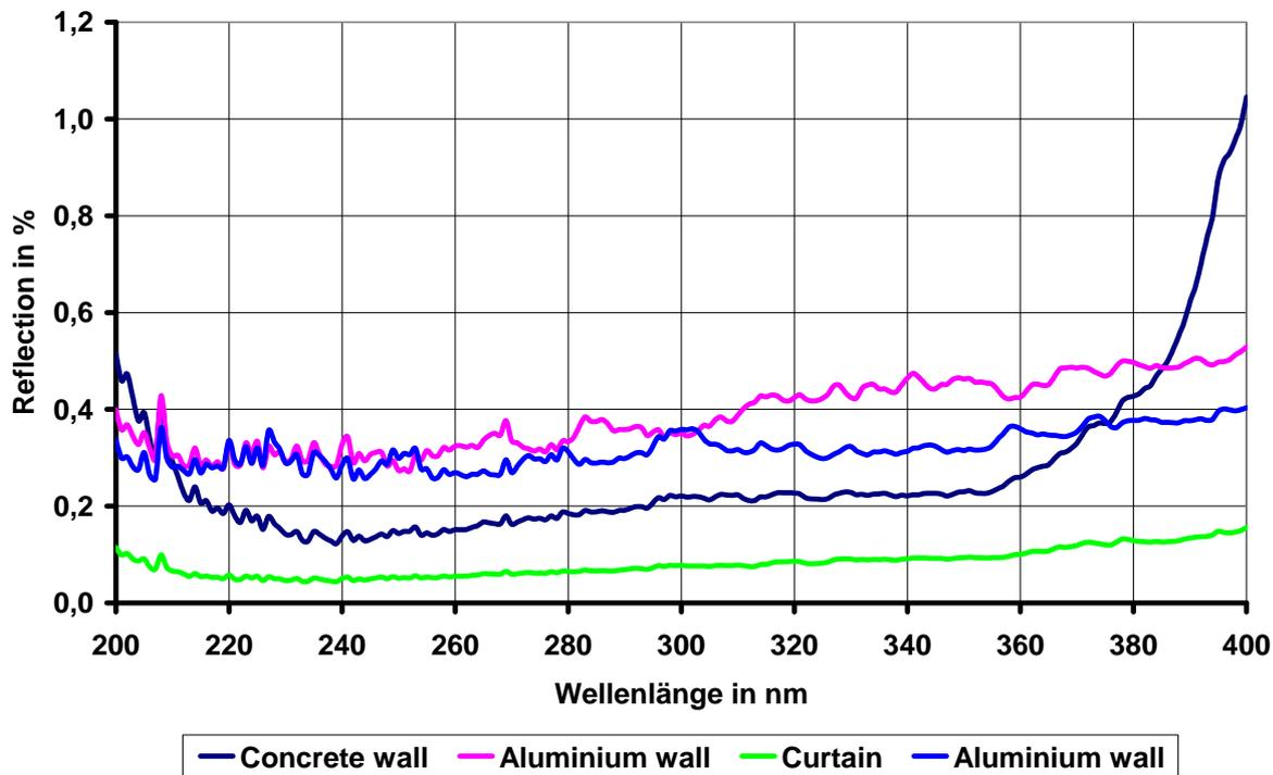
Figure 11: Spectral shares of reflected radiation during MMA welding with a welding current of 250 A
