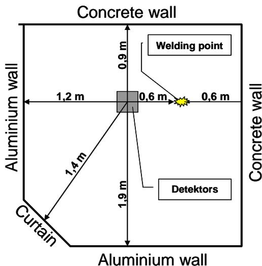
Figure 1: Design of the welding booth with the location of the welding point and the detectors. The arrows show the direction in which the detectors were pointing during measurements.
