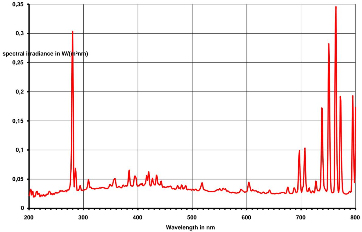
Figure 3: Radiation spectra during the TIG welding of Al (welding current 180 A)
