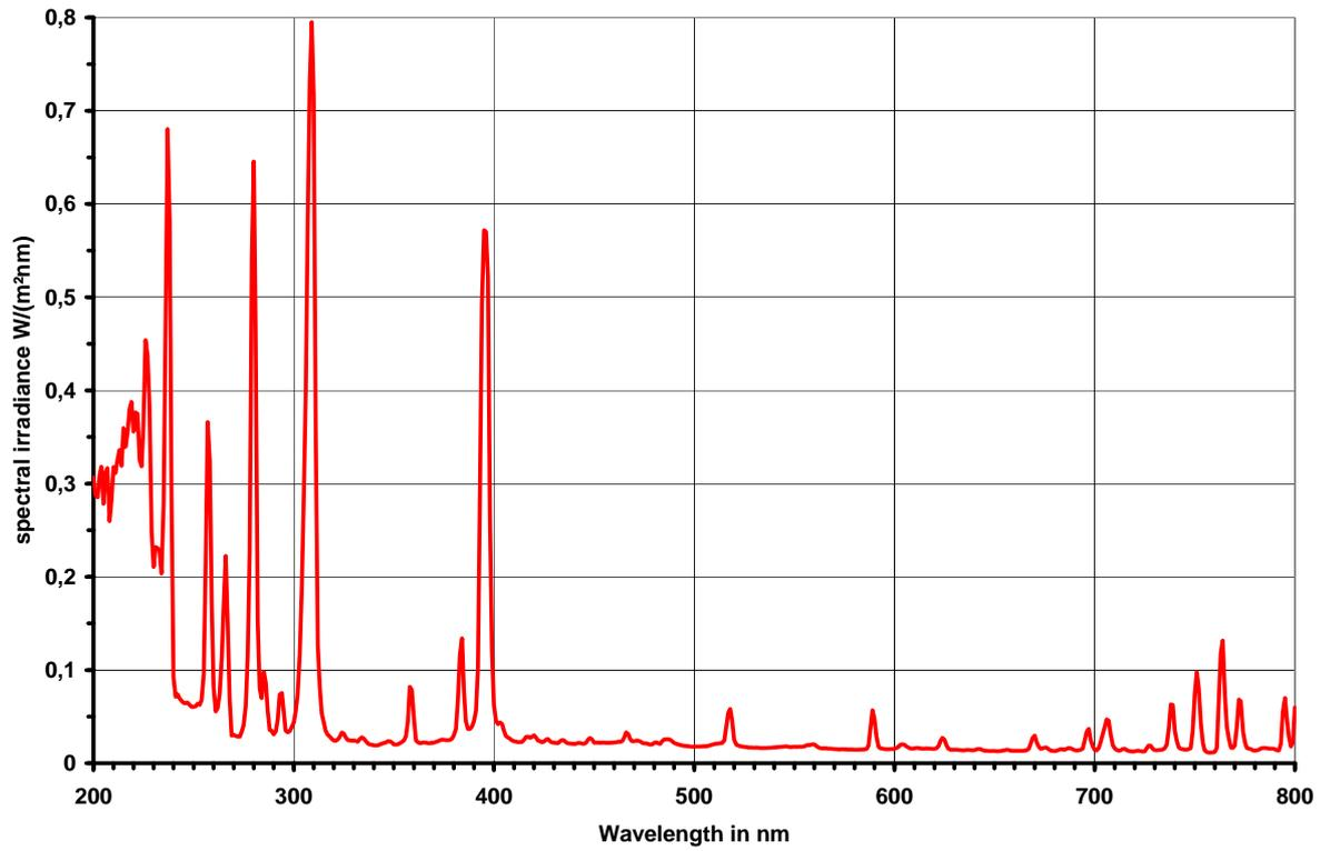
Figure 5: Radiation spectra during the MIG welding of Al (unpulsed welding current 180 A)
