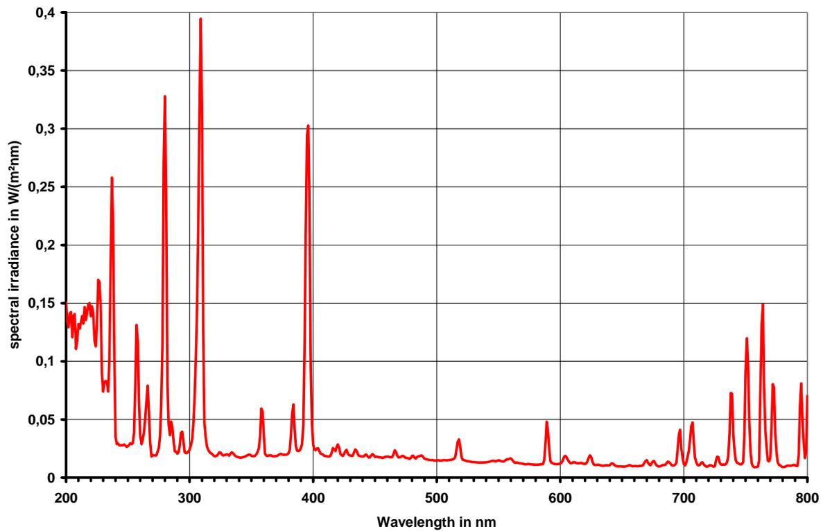
Figure 4: Radiation spectra during the MIG welding of Al (pulsed welding current 180 A)
