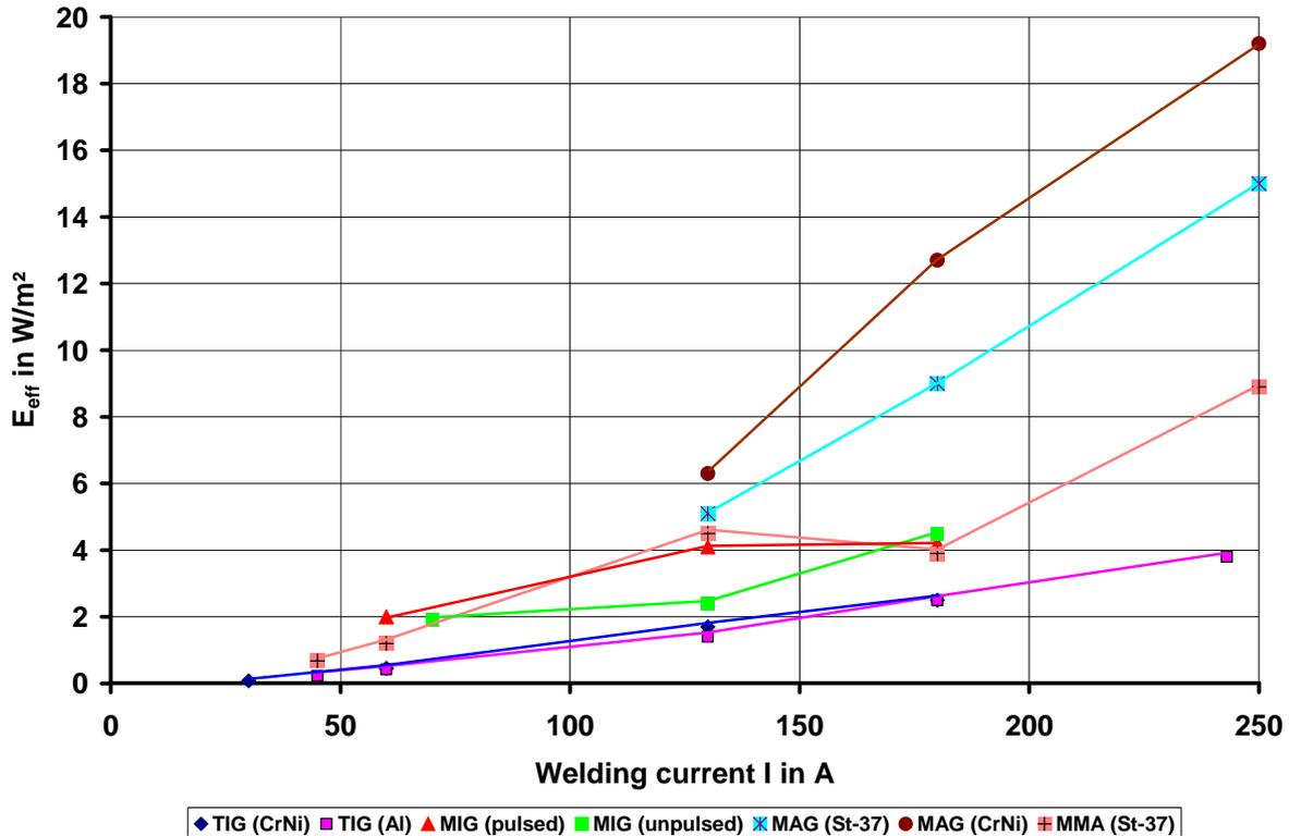
Figure 10: Effective irradiance at a 60 cm distance from the arc for different welding processes (radiometer readings)
