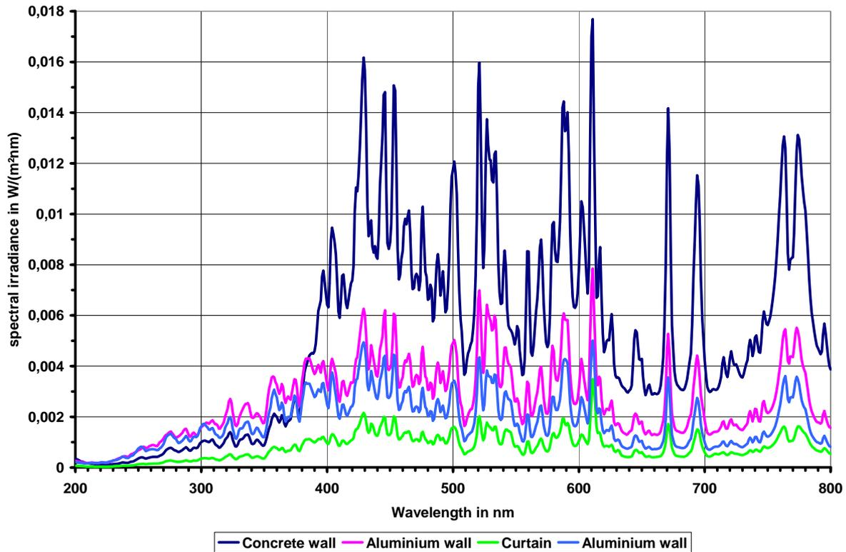
Figure 9: Radiation spectra of diffuse radiation during the MMA welding of St-37 (welding current 250 A)
