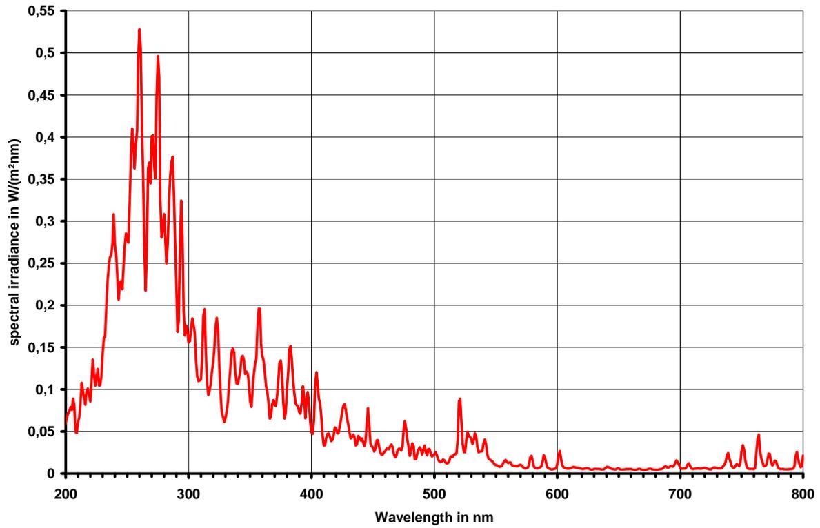
Figure 7: Radiation spectra during the MAG welding of CrNi (welding current 180 A)
