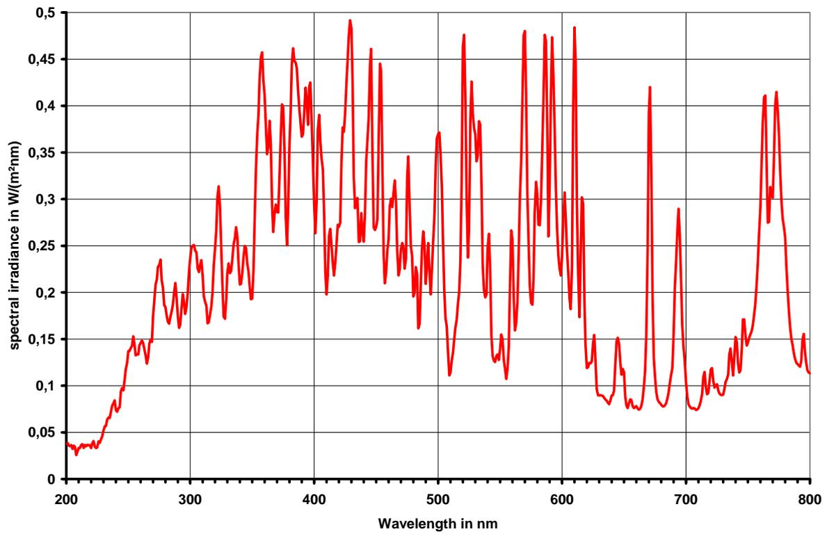
Figure 8: Radiation spectra during the MMA welding of St-37 (welding current 180 A)
