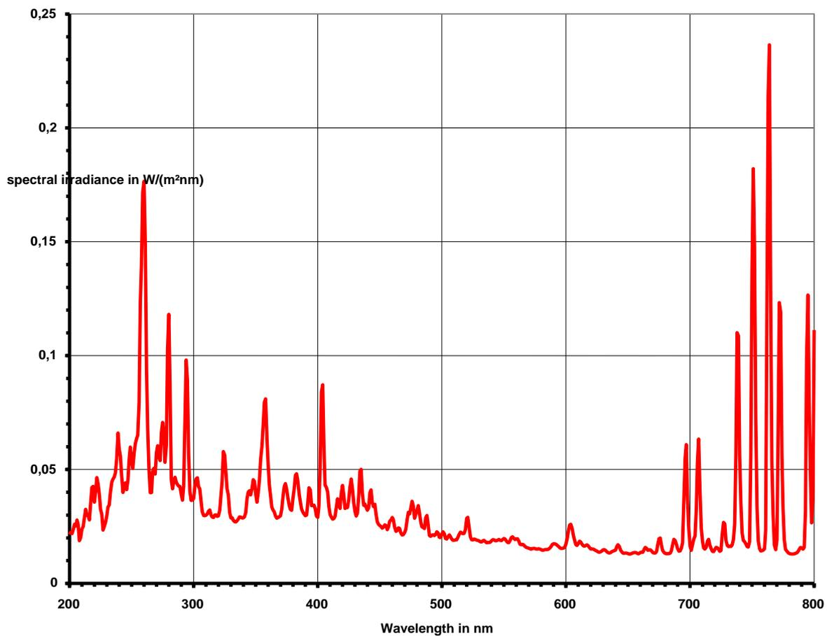
Figure 2: Radiation spectrum during the TIG welding of CrNi (welding current 180 A)
