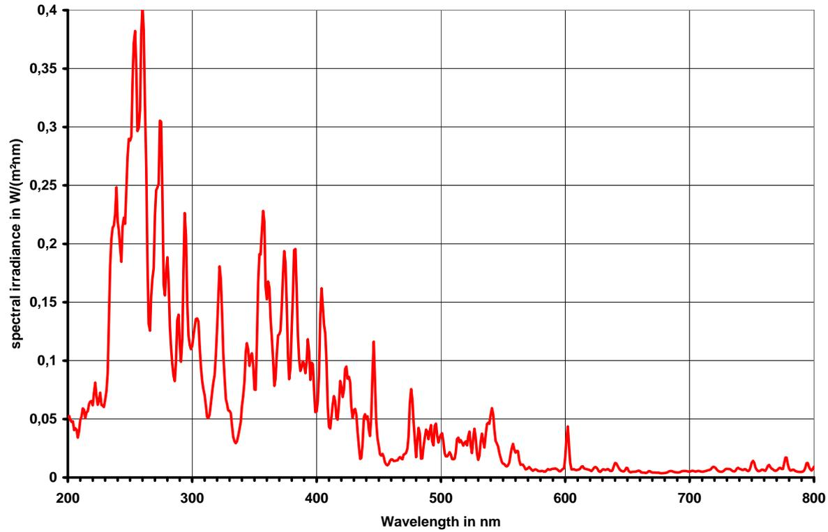
Figure 6: Radiation spectra during the MAG welding of St-37 (welding current 180 A)
