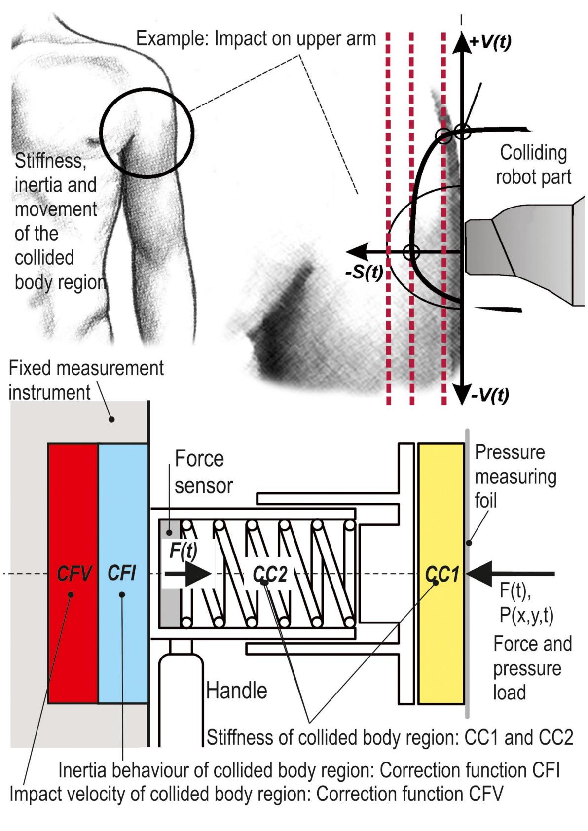
Schematic diagram of the KDMG-KOLROBOT force/pressure instrument for the testing of collaborative robots
