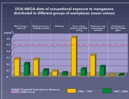
collected. For the majority of workplaces -with the exception of some welding activities-, more than 90 % of the measurement readings are below the threshold limit value (MAK-value) of 0.5 mg/m<sup>3</sup>. This is in accordance with a former preliminary investigation [4].
