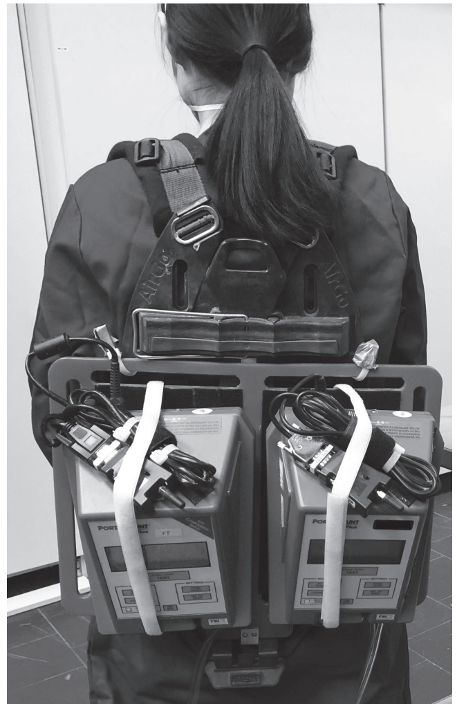
Figure 1. Subject equipped with the measuring instrument (PortaCount).
