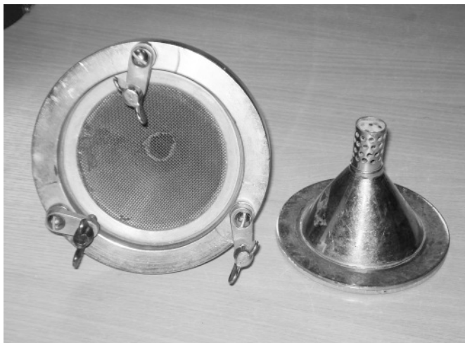
Figure 1. Double Cone (DC) sampling unit in use from 1959 until approximately 1971.
