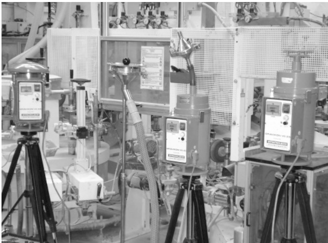
Figure 6. Left: On-site sampling with historic and modern sampling devices in a porcelain plant next to an isostatic pressing unit for plates. Right: Arrangement of sampling devices next to an isostatic pressing unit during on-site sampling.
