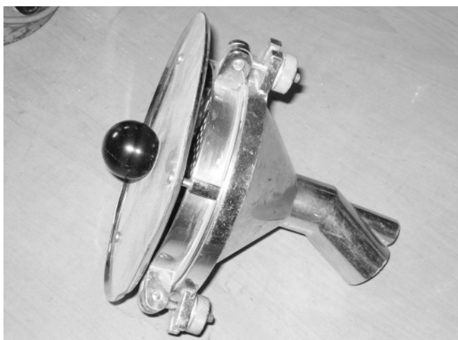
Figure 2. Gravikon WL 10/40 sampling unit in use from 1969 until approximately 1975.
