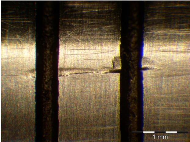
**Figure 9:** Microscopic image of a valve spool operated under poor conditions
