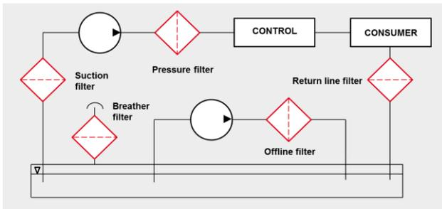
**Figure 3:** Diagram of filter types
