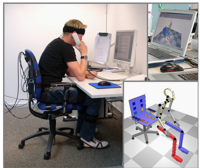
Measurement at a simulated office workplace in a laboratory environment; display in the WIDAAN software
