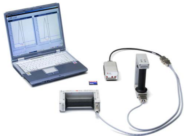
Left-hand and right-hand handle with data logger
