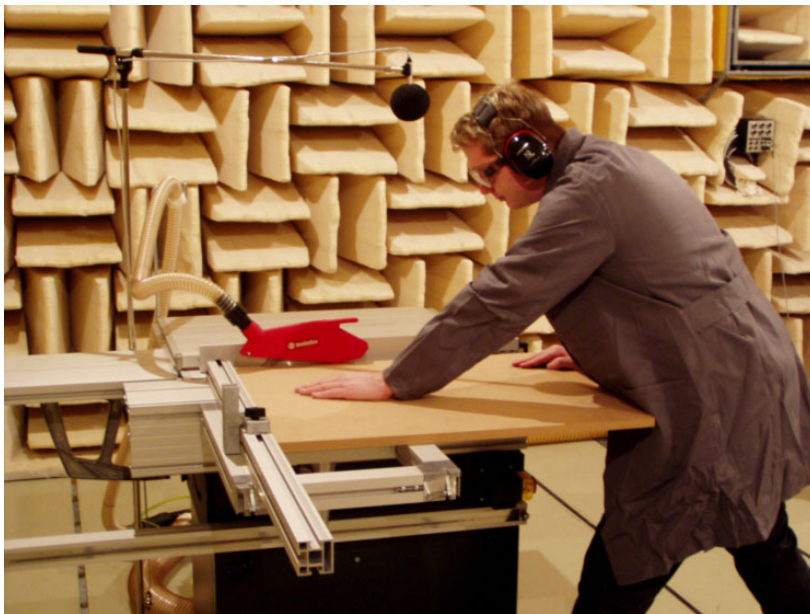
Illustration Measurement of noise emissions during sawing in the semi-soundproof chamber
