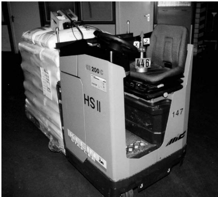
Illustration Pallet truck with driver's seat at 90° to the direc- tion of travel
